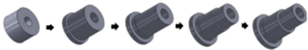
Fig. 1 Schematic representation of the steps in hot forging process to forge hollow shafts
